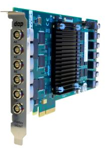
The PCIe's format takes flexibility to a higher level and addresses the industries growing support for this data interface. This solution enables users to install the FireSpy hardware in any modern PC that has at least one 4-lane PCIe slot available. This allows for installation of the FireSpy in developers existing PCs or installing the analyzer in a rugged field service laptop or lunchbox computer.
