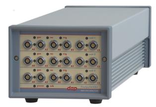
The FireSpy9x32bT has nine 1394 nodes connected to nine synchronized analysis engines. They are controlled by three dual core ARM processors running at 667MHz. Each node is connected to two 1394 ports. Both ports of each node are connected to a separate LEMO connector which was chosen over standard 1394 connectors for improved ruggedness.
