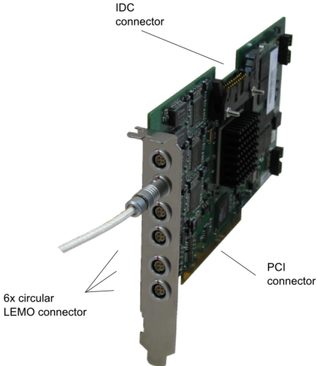
This FireSpy is a PCI card. It must be build into a PC.
