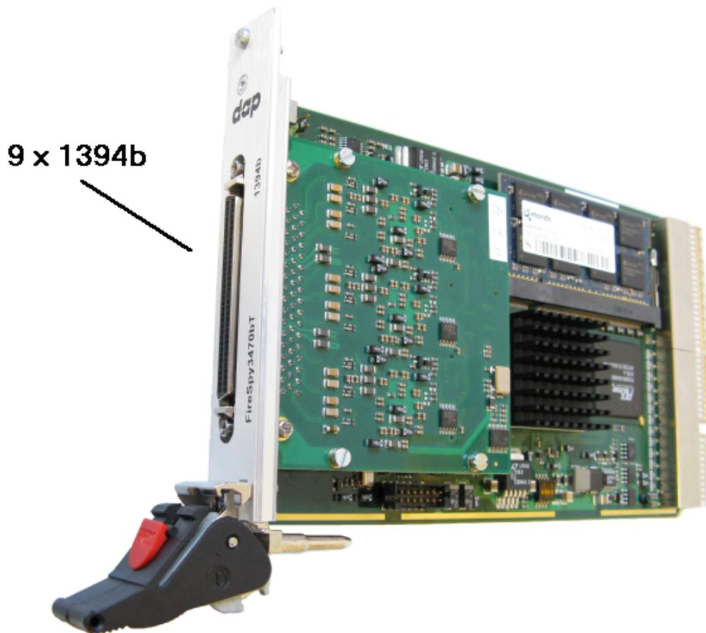
This FireSpy is a CompactPCI / PXI card, it must be fitted in a CompactPCI / PXI chassis.
