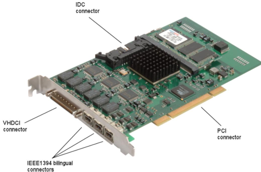
This FireSpy is a PCI card. It must be built into a PC.
