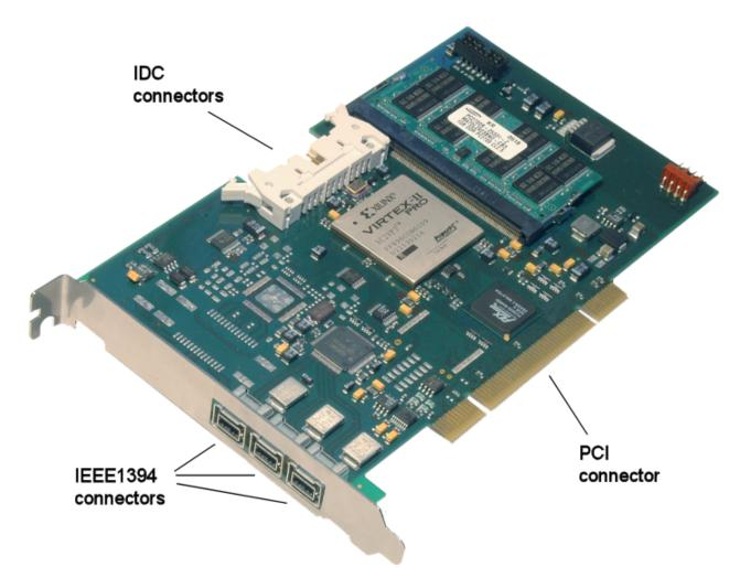
This FireSpy is a PCI card. It must be build into a PC.
