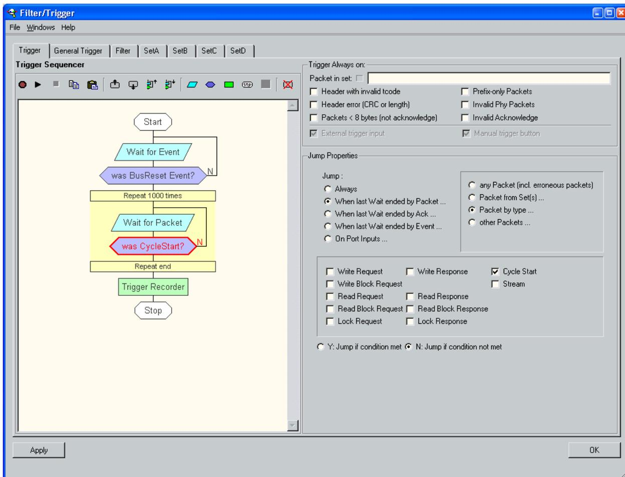
The most important part for the trigger settings is the **Trigger Sequencer**, see left pane in example above. Here you can graphically define a trigger program by adding items to the flow and change their properties. By executing the program you can generate a Recorder trigger when a particular sequence of packets or events has been detected.
