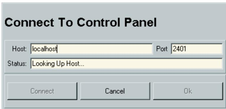
This dialog has two input fields, the host it must try to connect to and the port number. Because the communication between the Analyzer application and the client uses TCP/IP you need an IP address or a computername and a port number. The Analyzer application only accepts connection when the same icon is selected.
