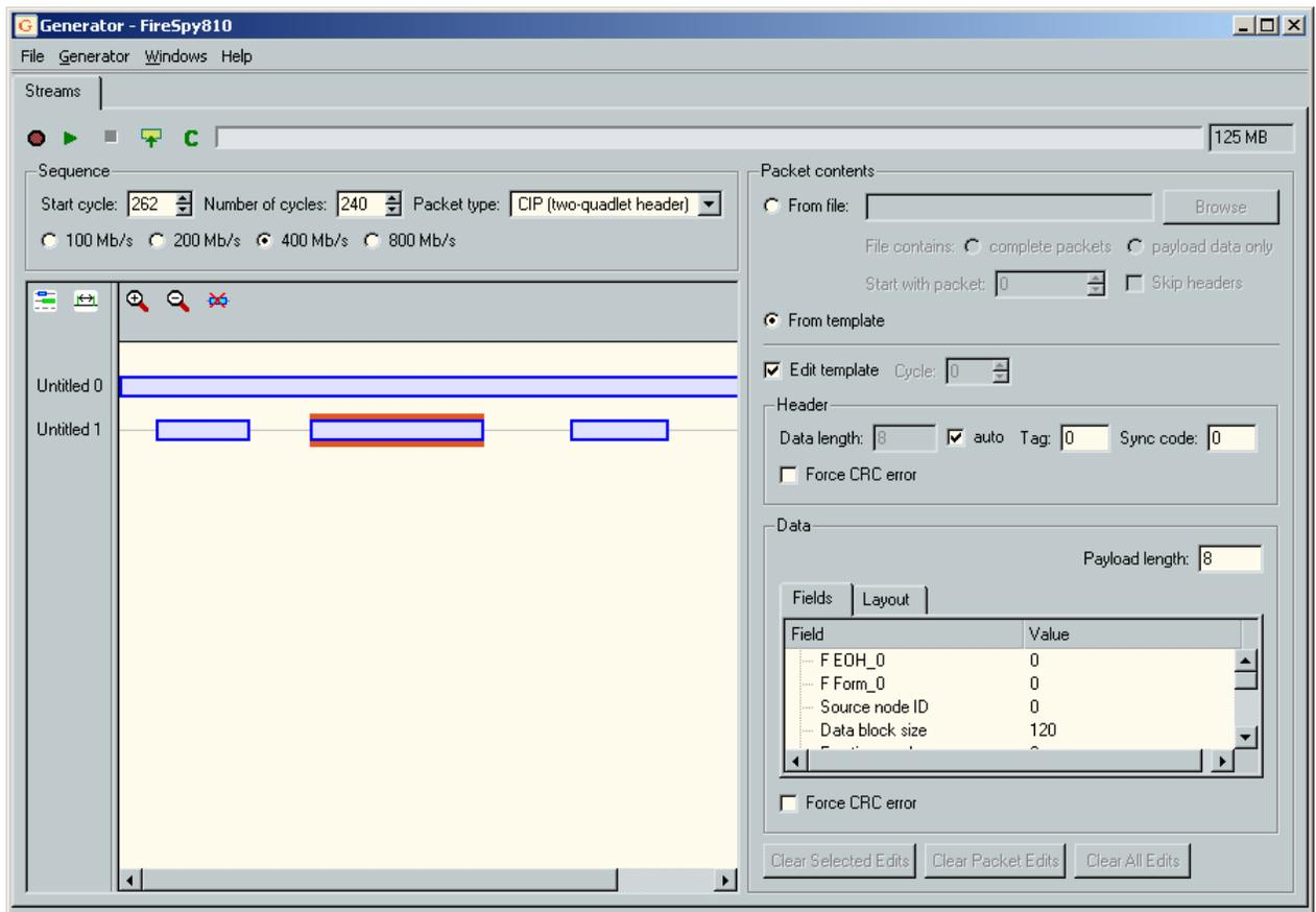
At the top of this window you can find the toolbar with buttons for starting, uploading and stopping the Generator. Before starting the Generator, you first have to upload the generator data to the Analyzer. This
