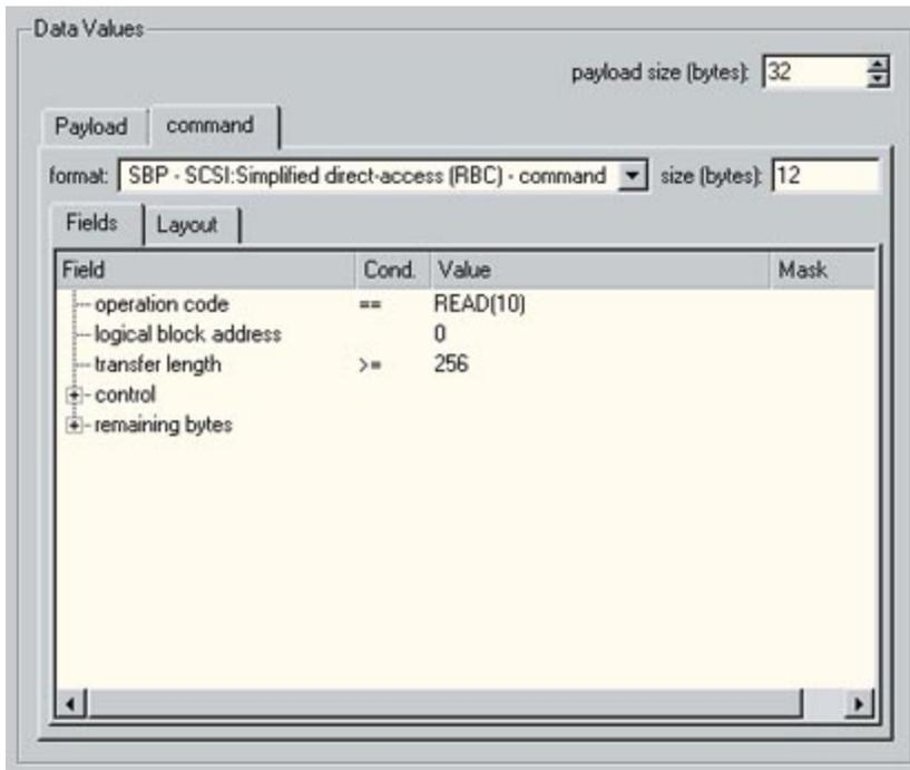
The selected format describes the commands for a 'Simplified direct-access (RBC)' unit. By choosing a value for the 'operation code' field, the format will automatically adjust to the format of the selected command.
