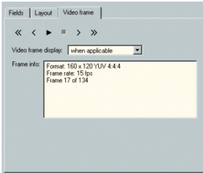
The tab displays information about the selected video frame and contains control buttons to select other video frames and to play back a sequence of video frames. The selected video frame is also displayed in a separate popup window shown below. The tab has a combo box that can be used to determine when the video window will be displayed. The possible choices are:
