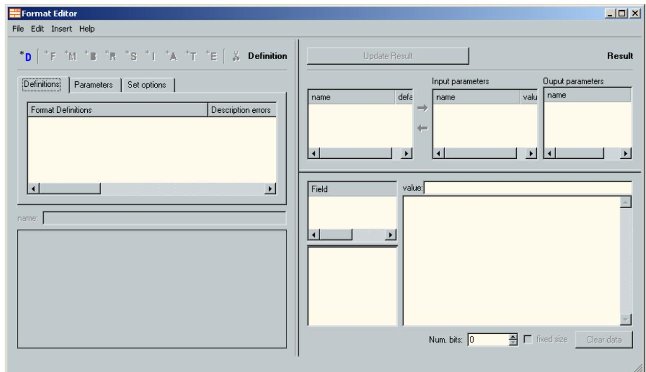
In the left pane of the window (Definition pane), you can create the definitions tree. The properties of a selected item is shown below the tree and can be changed there.
