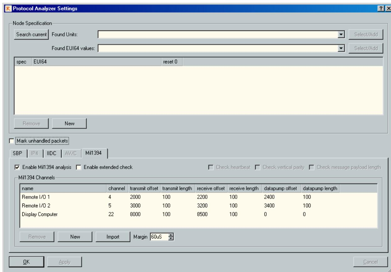
The information of the nodes, which support the Mil1394 Protocol, is to be added in the table 'Mil1394 Channels' of the Mil1394 tab page. Click on the Mil1394 tab to show the Mil1394 tab page on top.
