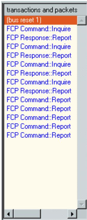
When an item is selected that consists of more than one packet or transaction, the items are highlighted in the 'transactions and packets' pane list with a gray bar (the selected item, which is also part of the item will still be highlighted with the usual selection color).
