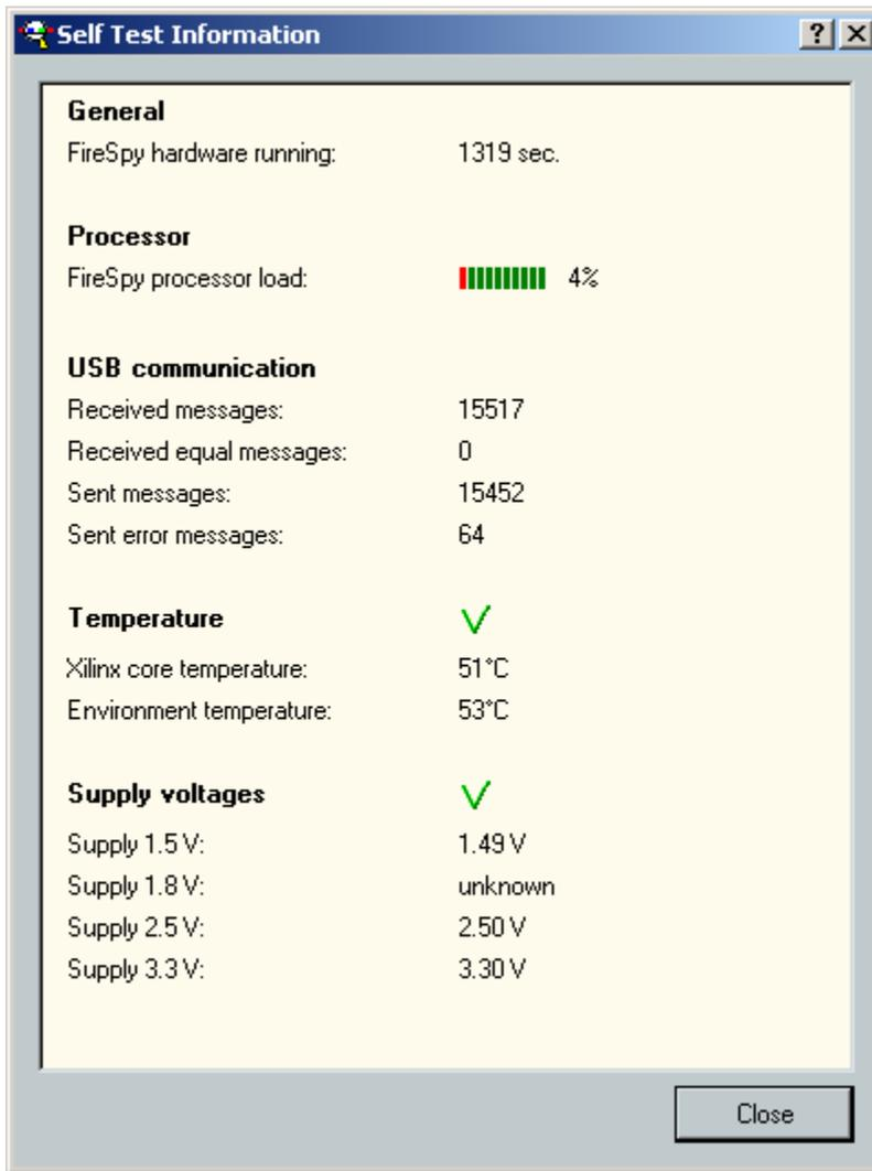
Selecting 'Analyzer Info' from the Help menu opens a window with information about the analyzer(s) currently in use:
