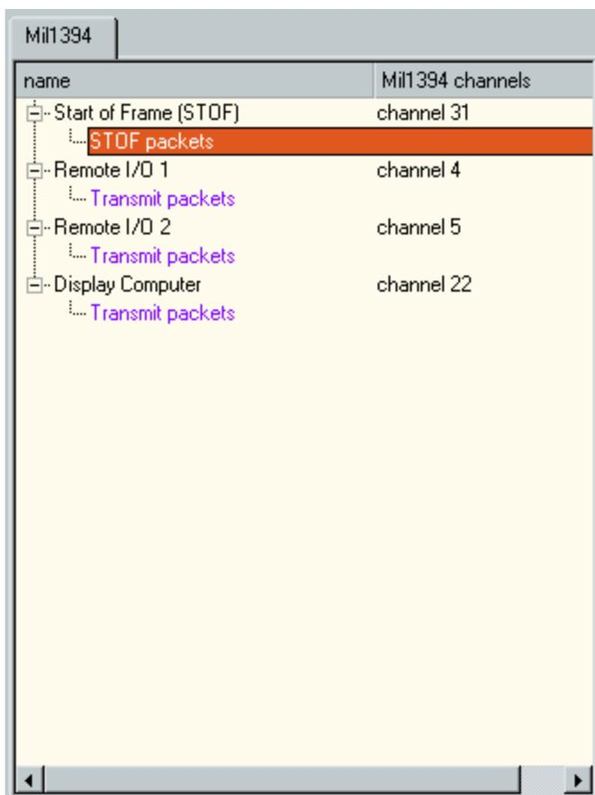
Root items (except the first root item) have four child items maximum. The child items represent the Transmit packets of the node, the Receive packets of the node, the DataPump packets of the node and the Unknown packets of the node. A packet is an Unknown packet if it can't be identified as one of the three Mil1394 packet types mentioned above. A child item of a root item is not displayed if not any Mil1394 packet in the 'transactions / packets' pane corresponds to the child item.
