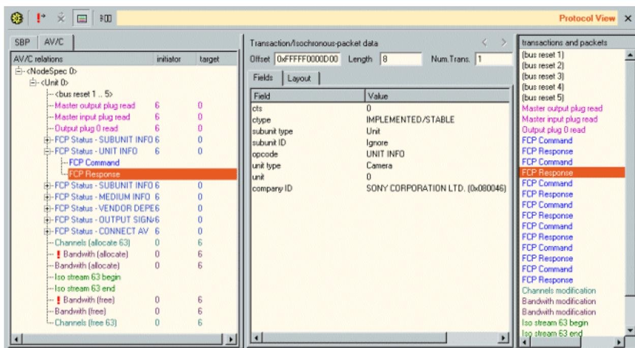
It displays the result in three different parts. At the right (transactions and packets), all found packets and transactions are displayed in the order they were detected on the bus. The left part (relations) shows the relation between these items. The transactions and packets belonging together (e.g. all transactions that form a single FCP command) are grouped into tree items and these items are displayed hierarchically in the 'relations' pane. In this tree you will find for instance:
