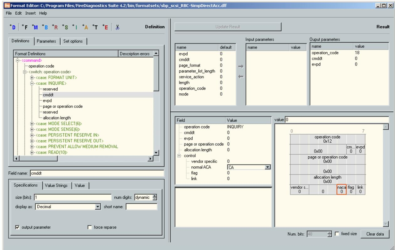
In the 'Definition' pane you see the format definitions tree. The name of the first definition is 'command'. It starts with a field with name 'operation code'. This item is selected, so the properties of this 'Field' item are displayed below. It is a 8 bit field of type 'Hexadecimal'.
