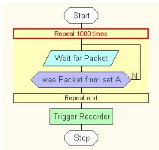
Now the flow does something meaningful: the Recorder will be triggered when 1000 packets have been detected that fits the description for packet setA. Below the Repeat item will be described in more details.
