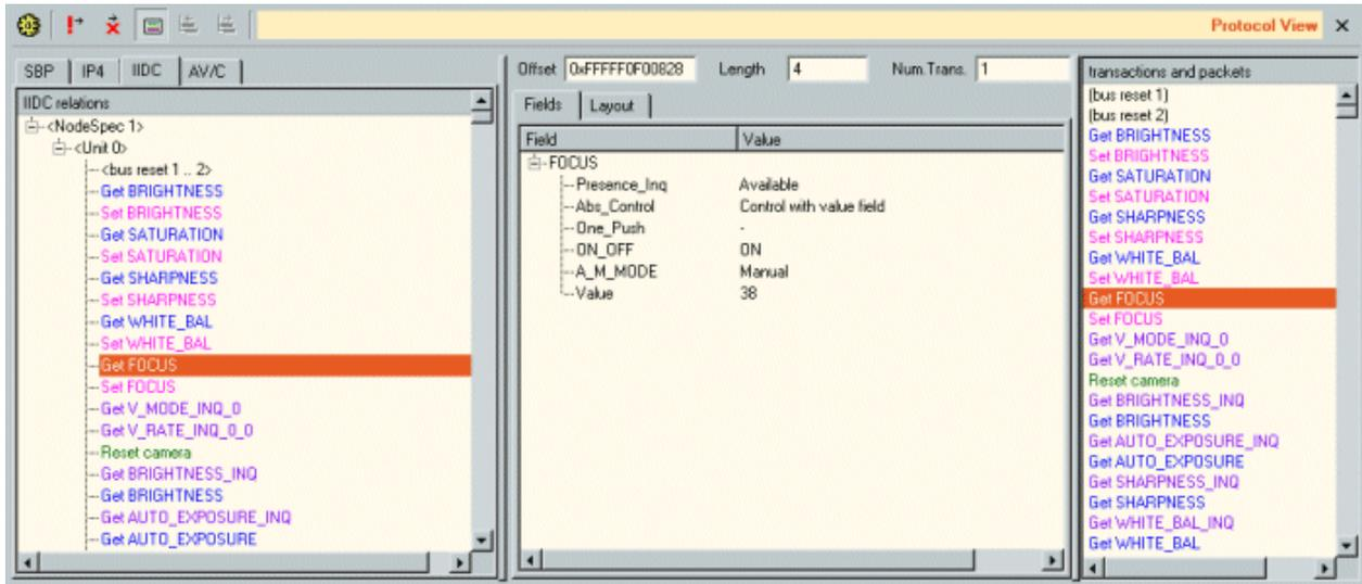
It displays the result in three different parts. On the right (transactions and packets), all packets and transactions found are displayed in the order they were detected on the bus. The left part (relations) shows the relation between these items in a hierarchical tree. The transactions and packets belonging together are grouped into tree items and these items are displayed hierarchically in the 'relations' pane. In this relations tree you will find for instance:
