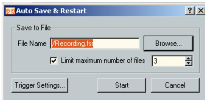
Using this dialog you can select location and 'BaseName' for the recordings, number of the recordings and configure trigger.
