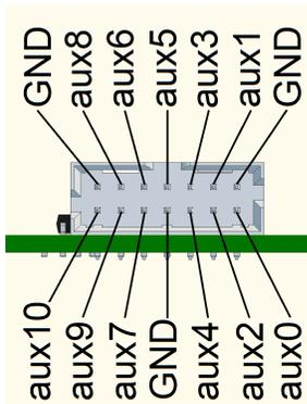
This 14 pins connector has the following signals:
