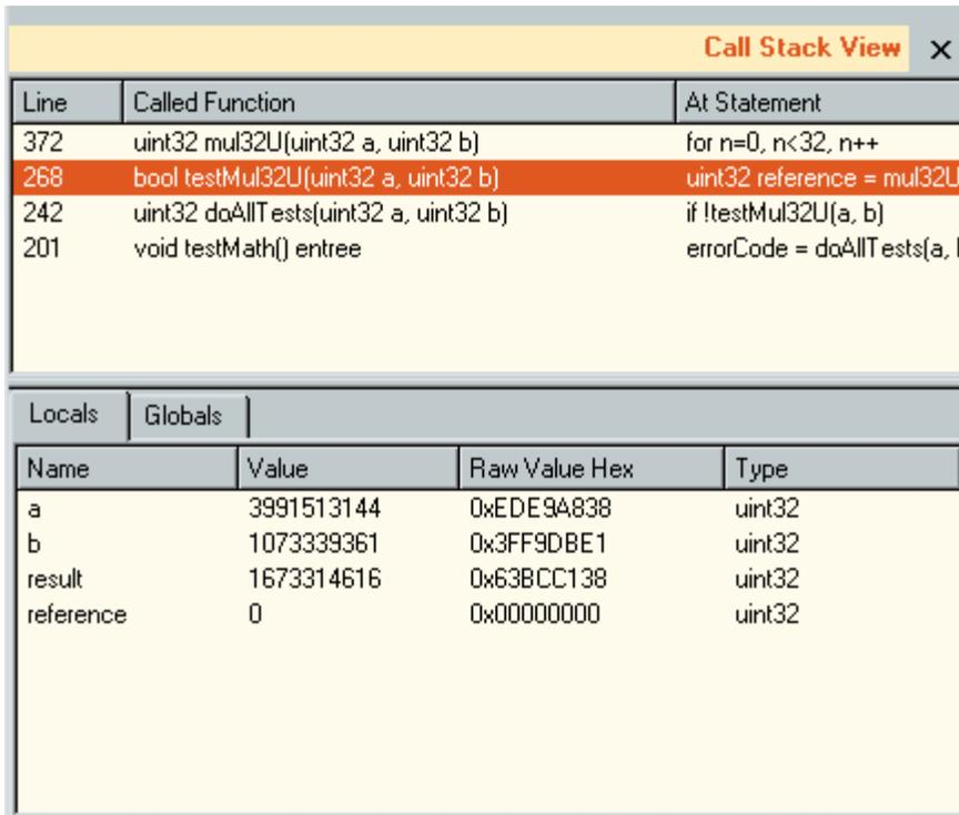
The Call Stack View displays symbol and function-call information for the process that is currently selected in the Process View. If the Process View has no selection, this view will be empty.
