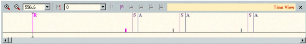
In this example a Bus Reset occurred, followed by two Phy-SelfID packets. After the second SelfID packet there is for some time no packet, resulting in the Subaction Gap and Arbitration-Reset Gap events. Then a cycle-start packet is transmitted and again a while nothing, resulting in the Subaction Gap and Arbitration-Reset Gap again, etc.
