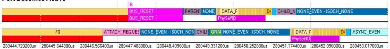
After the port detects making it active will not result in a loop, it sends an ATTACH\_REQUEST which is responded with a BUS\_RESET control. (See Chapter 14.7.9 and 14.7.10 of the specification).
