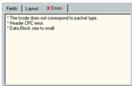
If one or more fields or data is missing (like in the case of 'Data-Block size too small' error above) the 'Field' and 'Layout' pages will also reflect the error by displaying the missing parts in red. Likewise, when there is too much packet data, the parts that are too much are also displayed red in the 'Fields' and 'Layouts' pages.
