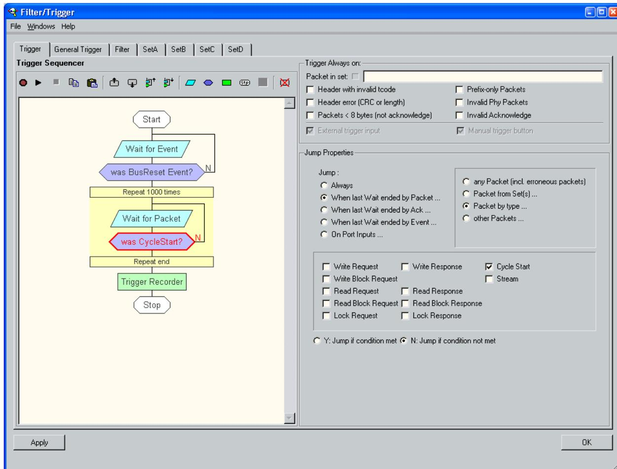
In this example a little more complex Trigger Sequencer program flow is used. And a cyclic pre-trigger buffer has been enabled that will never use more than 25% of the total Recorder memory. We will discuss the different part of this page in more details below.
