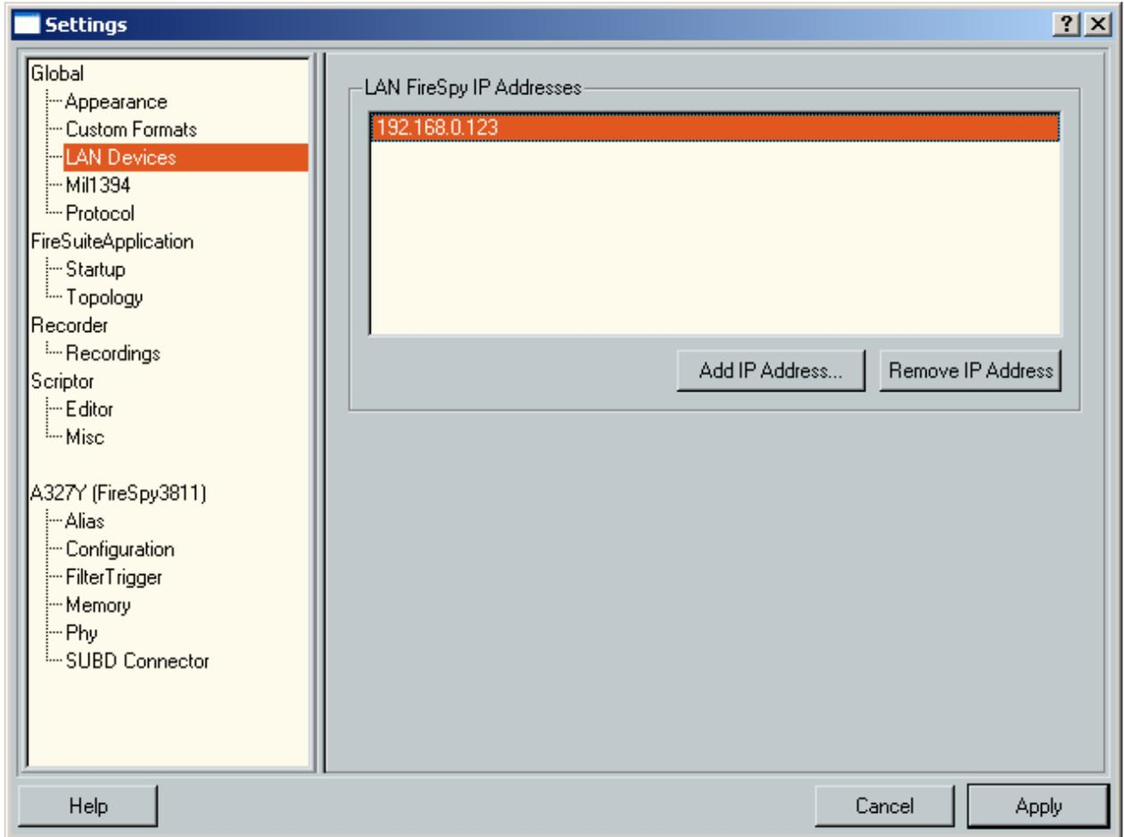
The FireDiagnosticsSuite can use Analyzers connected via ethernet after they are configured with the EthernetConfig tool. To have the application look for an ethernet device, add its IP Address in the box above.
