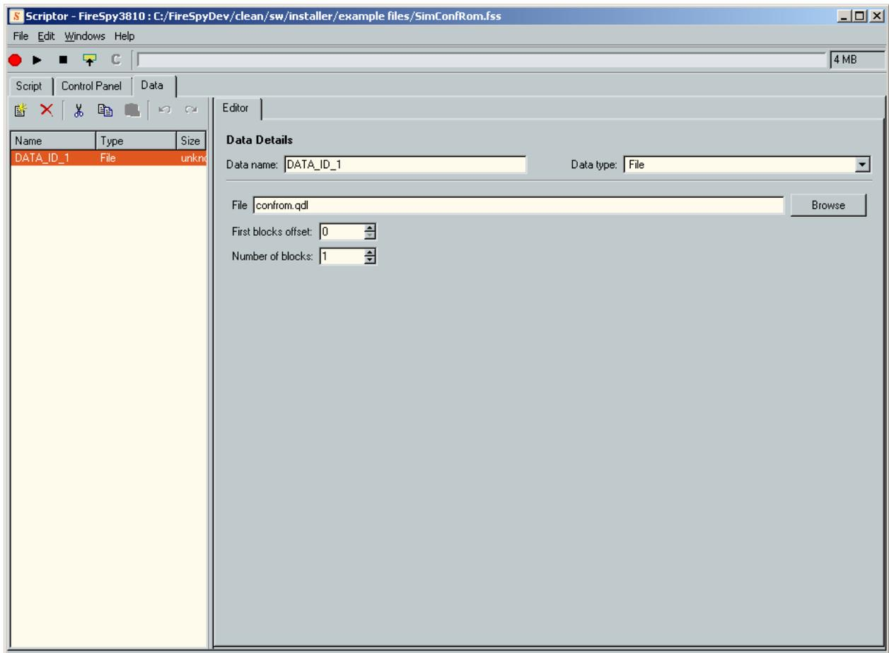
Note that the data is read from file during script upload from the specified file. When the script is running on the Analyzer, the file data is already in Analyzer memory.
