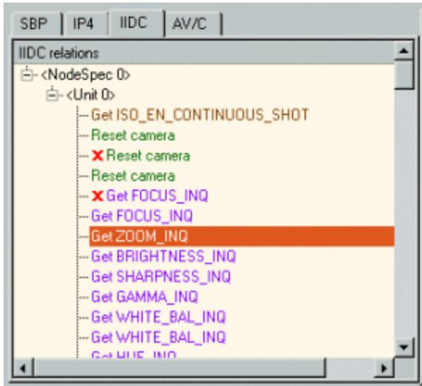
For each found or manually specified NodeSpec there will be a root item in the tree (NodeSpec 0 above). For information about NodeSpec's, see 'IIDC-Protocol Settings' below. For each found or manually specified Unit, there will be a Unit item inside the corresponding NodeSpec (Unit 0 in NodeSpec 0 above).
