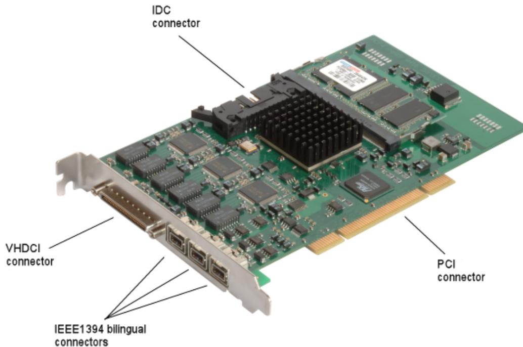
This FireSpy is a PCI card. It must be build into a PC.
