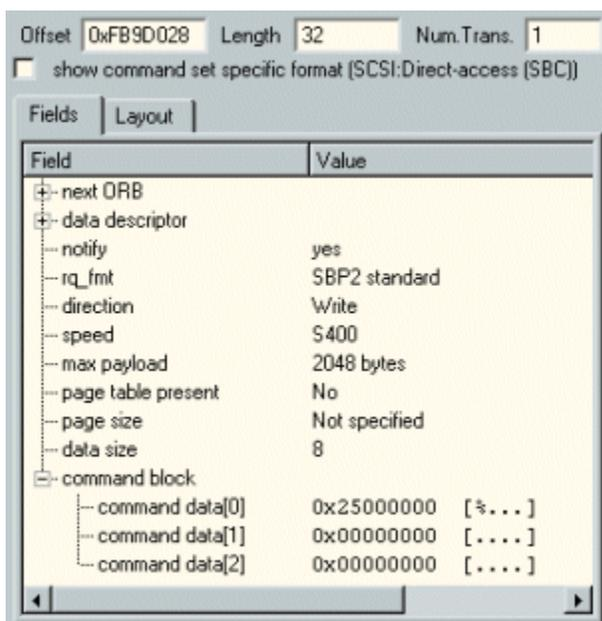
Without the option checked (example above), all the fields of the item are listed, including the command-set-specific part ('command block' in the example above). Note however, that the command-set-specific part is not formatted in this case. It is just the SBP definition of the ORB block.
