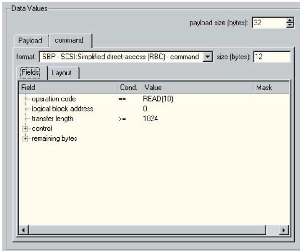
Decimal and hexadecimal numbers can be entered decimal or hexadecimal. For fields with symbolic values, a combo box will be displayed when clicking on the value so that a value can be chosen. You can change this behaviour by selecting an other display form (overruling the automatic form) using the right mouse button as described below.
