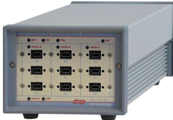
The FireSpy3x30xx has three 1394 nodes connected to three synchronized analysis engines. They are controlled by a dual core ARM processor running at 667MHz. Each node is connected to three 1394 ports. All ports of each node are connected to a separate IEEE-1394 connector with screw mount holes which was chosen over standard 1394 connectors for improved ruggedness.
