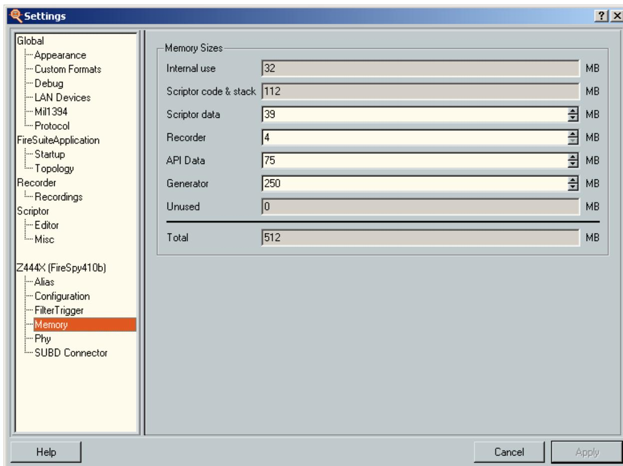
The total memory is shown as the last item in the list. Part of the internal memory is allocated by the Analyzer itself. This allocation is fixed and cannot be changed. The following fixed memory allocations exist:
