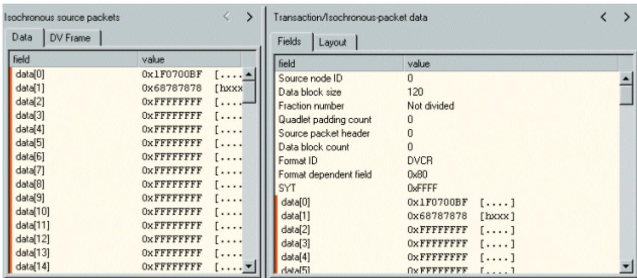
In this example, the data in one isochronous packet corresponds, again, exactly to one source packet (DV
