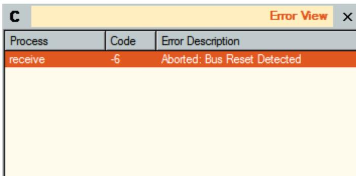
Many of the Scriptor library functions will return a negative value in case of error. When running in debug mode, these negative return codes will always be sent to the debugger, even if the script does not contain any return value checking.
