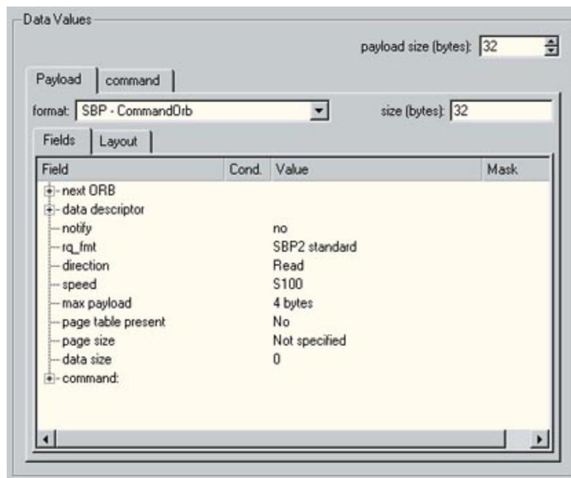
The fields in the table show the fields for the payload of this packet format. You can put conditions on these values just as could be done with the header fields. If the format of a packet depends on the value of one of its fields, the format will automatically be adjusted if you change the value of that field.
