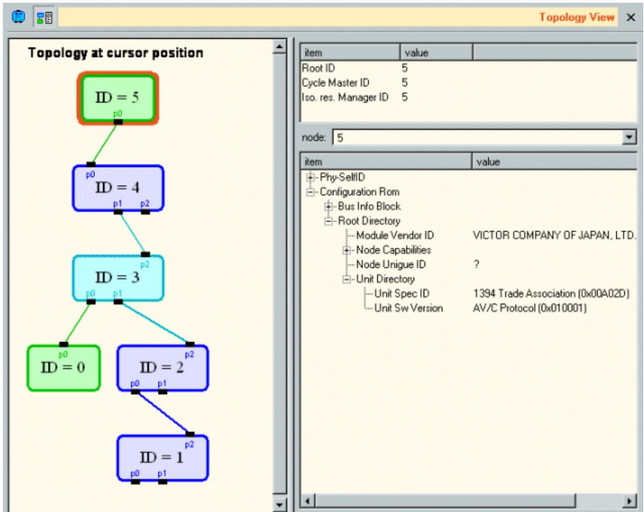
The extra node information consists of information from the selfIDs from this node and information from the Configuration Rom of this node. For values that could not be found (no read of the corresponding Configuration ROM address recorded) a '?' will be displayed.
