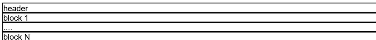
The header consists of two 32-bit values, one file identification and one version number.
