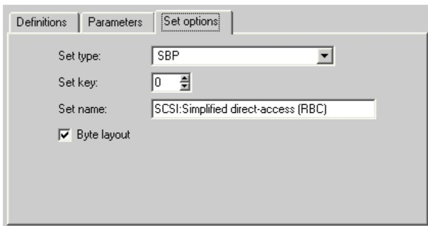
It defines an SBP (SBP2) Set type for a Direct-access (SBC) device. The Set type and Set name and sometimes the Set key are used by the Analyzer to find the correct format definitions. How these fields need to be filled in depends on the protocol the format set is used for. For details on this, see the corresponding document file (e.g. the ['Editing SBP2 formats'](#) section for more details on these Set options for the SBP2 protocol).
