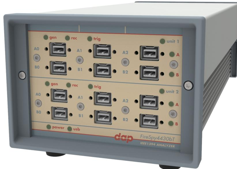
The FireSpy4x30xx has four 1394 nodes connected to four synchronized analysis engines. They are controlled by two dual core ARM processors running at 667MHz. Each node is connected to three 1394 ports. All ports of each node are connected to a separate IEEE-1394 connector with screw mount holes which was chosen over standard 1394 connectors for improved ruggedness.
