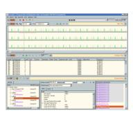
The *Recorder* is the main tool for data traffic capturing and analysis. Running all in HW/FW it guarantees precise time measurement, reliable data capture, instantaneous triggering and enough memory for even very complex analysis tasks. It contains several display views, which can all be switched on or off individually.
