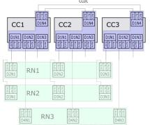
However, the above is only an implementation variant. A 4-node **FireTrac**<sup>®</sup> can also be used to simulate single branch bus behavior (left and middle) or mixed CC/RN situation in double redundancy (right).
