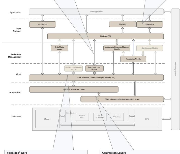
FireStack® Core forms the engine of the software stack. Core processes all functions such as user notification, interrupt event handling, background processing tasks, packet (isochronous and asynchronous) receive and transmit, memory allocations, timers, etc.. FireStack® Core is not specific to any device or OS and is designed to run on top of the Link and OS Abstraction Layers.
