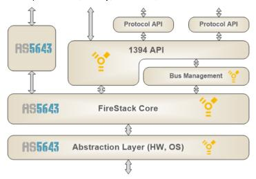
Conceptually, FireStack<sup>®</sup> addresses all these issues. It complies with IEEE1394 requirements as well as select higher protocol layers e.g. IIDC). And as the only product in the market it natively supports AS5643 features and functions. Due to the time critical aspects of that AS5643 protocol the AS5643 portion of FireStack<sup>®</sup> is only supported when running on top of an LLC with embedded AS5643 HW support (see FireLink<sup>®</sup> and FireTrac<sup>®</sup>).
