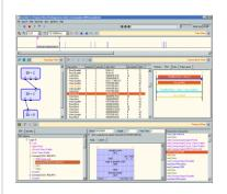
The **Recorder** is the main tool for data traffic capturing and analysis. Running all in HW/FW it guarantees precise time measurement, reliable data capture, instantaneous enough and triggering for even very memory complex analysis tasks. It contains several display views, which can all be switched on or off individually.
