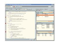
The **Scriptor** permits the definition of C-like scripts to control almost anything on the FireSpy, including sending and receiving of packets. It is the preferred tool for the generation of individual asynchronous packets, asynchronous sequences and the simulation of entire handshakes.
