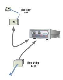
The FireStealth requires a pass-through wiring. Due to its symmetrical but entirely passive data pickup logic it has to be connected between other devices on the bus. Contrary to other FireSpy bus analyzers it cannot be in a leaf node position.
