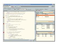
The Scriptor permits the definition of C-like scripts to control almost anything on the FireSpy, including sending and receiving packets. It is the preferred tool for the generation of individual packets. asvnchronous asynchronous sequences and the simulation of entire handshakes.
