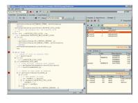
The Scriptor permits the definition of C-like scripts to control almost anything on the FireSpy, including sending and receiving packets. It is the preferred the tool for generation of individual asynchronous packets. asynchronous sequences and the simulation of entire handshakes.
