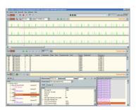
The *Recorder* is the main tool for data traffic capturing and analysis. Running all in HW/FW it guarantees precise time measurement, reliable data capture, instantaneous triggering and enough memory for even very complex analysis tasks. It contains several display views, which can all be switched on or off individually.
