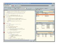
The **Scriptor** permits the definition of C-like scripts to control almost anything on the FireSpy, including sending and receiving of packets. It is the preferred tool for the generation of individual asynchronous packets, asynchronous sequences and the simulation of entire handshakes.
