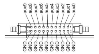
This 20 pins conector has the following signals:
