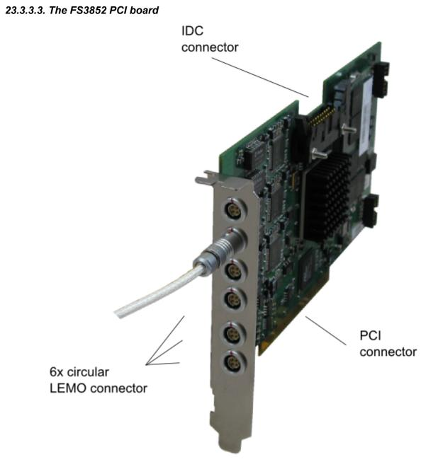
This FireSpy is a PCI card. It must be build into a PC.
