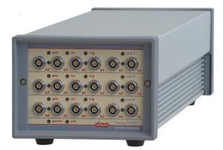
The FireSpy9x32bT has nine 1394 nodes connected to nine synchronized analysis engines. They are controlled by three dual core ARM processors running at 667MHz. Each node is connected to two 1394 ports. Both ports of each node are connected to a separate LEMO connector which was chosen over standard 1394 connectors for improved ruggedness.
