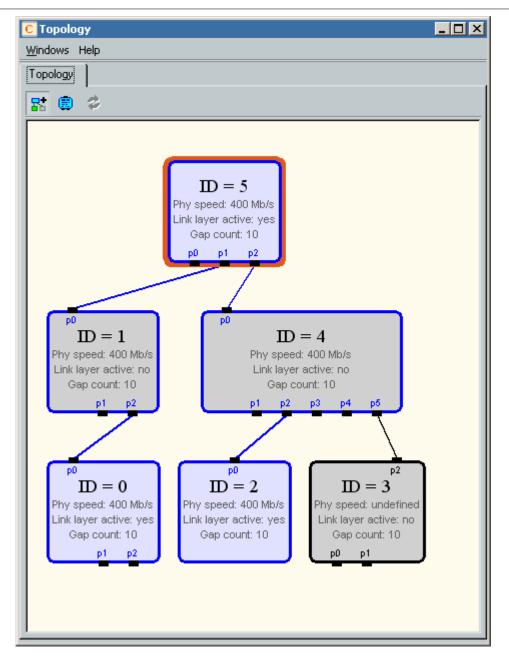
Whenever configuration of the FireStealth is done after configuration of the 1394b bus, the FireStealth will have missed the IEEE 1394b bus configuration and will not be able to gather the bus topology information.
