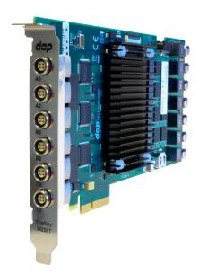
The PCIe's format takes flexibility to a higher level and addresses the industries growing support for this data interface. This solution enables users to install the FireSpy hardware in any modern PC that has at least one 4-lane PCIe slot available. This allows for installation of the FireSpy in developers existing PCs or installing the analyzer in a rugged field service laptop or lunchbox computer.
