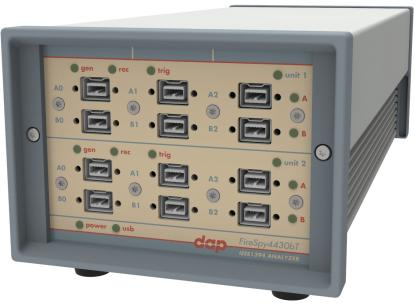
The FireSpy4x30xx has four 1394 nodes connected to four synchronized analysis engines. They are controlled by two dual core ARM processors running at 667MHz. Each node is connected to three 1394 ports. All ports of each node are connected to a separate IEEE-1394 connector with screw mount holes which was chosen over standard 1394 connectors for improved ruggedness.
