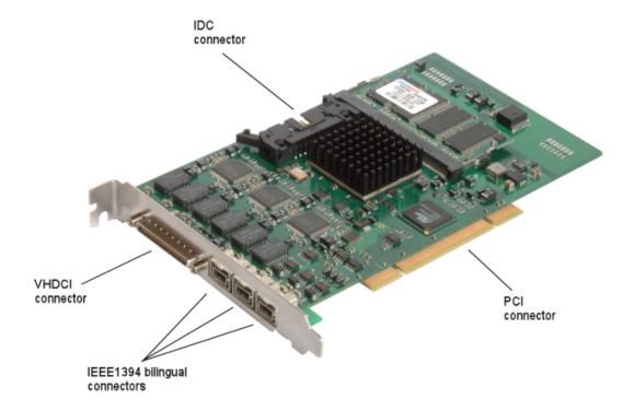
This FireSpy is a PCI card. It must be build into a PC.
