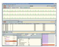
The *Recorder* is the main tool for data traffic capturing and analysis. Running all in HW/FW it guarantees precise time measurement, reliable data capture, instantaneous triggering and enough memory for even very complex analysis tasks. It contains several display views, which can all be switched on or off individually.
